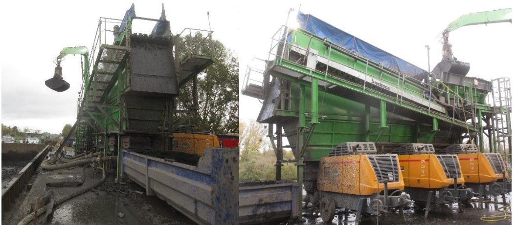
Starscreen with 1.7 m screen width as a protective screen for a sewer excavation feed pump. Screening is implemented at a diameter of 60 mm and a maximum length of 180 mm. The fine fraction is delivered 500 - 800 m by 3 concrete pumps.
