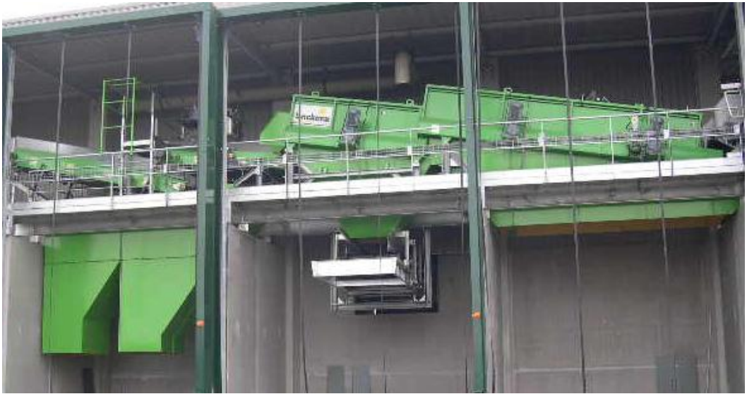
2 starscreendecks in series with an electric drive.
