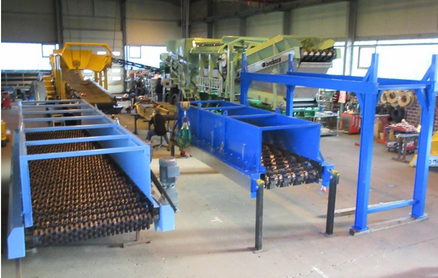
Assembly hall for the production of stationary and mobile star screens at the Twist site.
