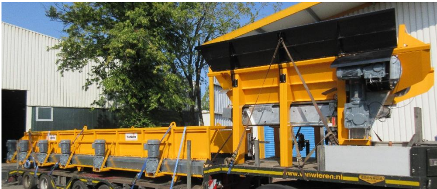
The starscreens are manufactured with an electric or hydraulic drive. In addition, Backers offers many custom-made products.
